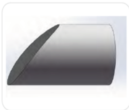
Cleave lensed fiber
